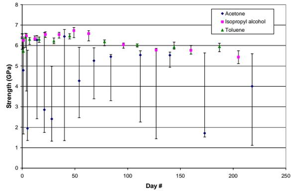
Figure 2: Acrylate fiber aging behavior in chemicals
