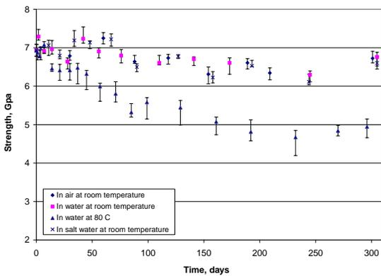
Figure 5: Aging behavior of polyimide fiber in water
