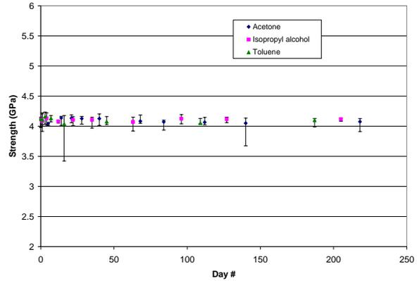
Figure 8: Aging behavior of carbon-polyimide fiber in chemicals
