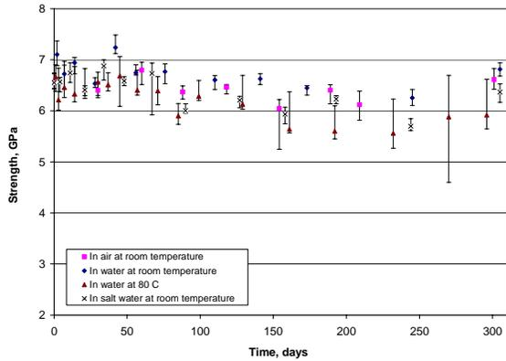
Figure 3: HCS fiber aging behavior in water
