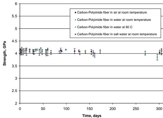
Figure 7: Aging behavior of carbon-polyimide fiber in water
