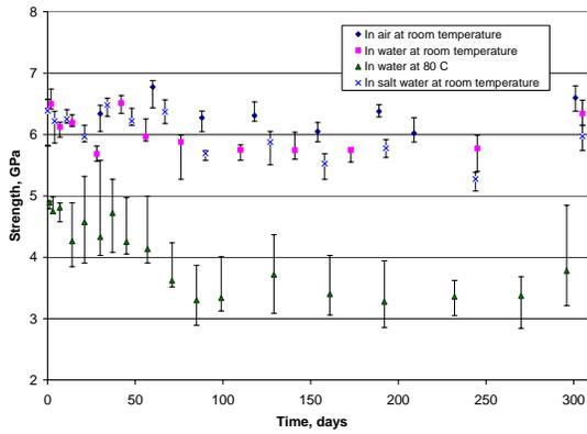
Figure 1: Acrylate fiber aging behavior in water
